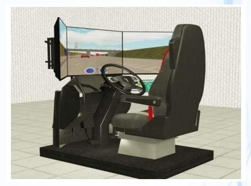
Mid-range Truck Driver Training & Research System with top-of-the-range software, 2DOF or 3DOF fully motion Budget model of AS 1000-T
